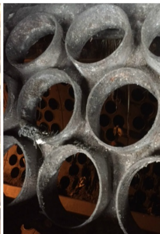
Metal rings fitted on the outside of the trommel help keep the holes clear of waste.
