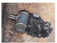
Images: Examples of 'zombie' batteries - one ignited at Hills recycling facility and the other in a waste collection vehicle but were both extinguished before causing any serious harm.
